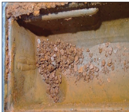
Rust sediments in the radiator prevent proper flow and create over-pressure & over-heating
