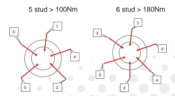
Warning: Failure to follow this tightening sequence can cause the drum to distort.
