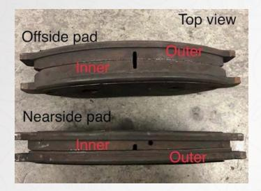
This issue had spanned over a few months. It had started with the owner of the vehicle purchasing the vehicle and requesting for the brakes to be replaced. A few months after the brakes were replaced the owner reported of squealing noises at low speeds as well as a burning smell. Upon removing the front discs and pads, they discovered that the NSF outer (or finger side pad) had worn down considerably more than the inner pad.
