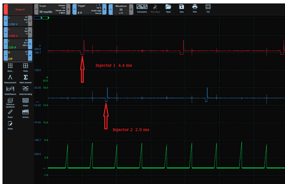
A scope trace showed the injector firing times were shorter for cylinders 2 and 3 when the engine was at operating temperature
