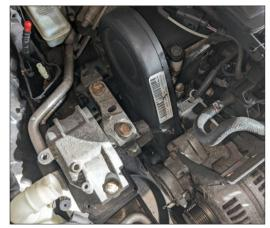
The noisy water pump was replaced, and a new tensioner fitted before fitting a new belt and boxing things up
