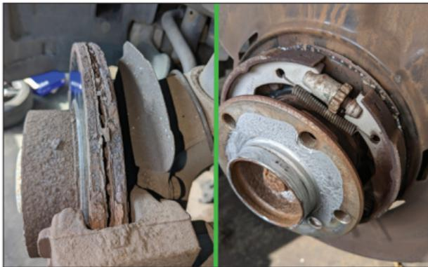
**The brake discs were badly corroded and the pads and shoes needed replacement**
