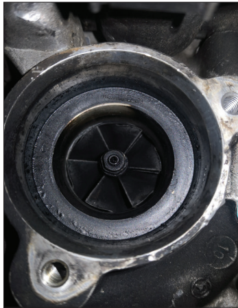
The smaller, high pressure turbo was easier to replace than the larger, low pressure turbo
