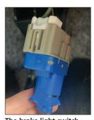
The brake light switch was the simple solution to the problems of the ABS and cruise control not operating
