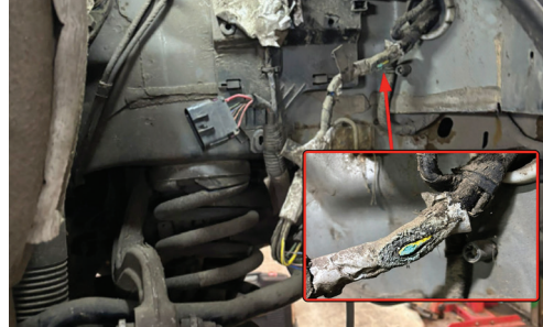
Wiring to the EPB Motor was damaged, at arrow
