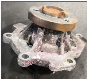
Coolant staining was evident on the water pump
