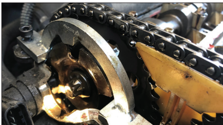
A setting tool is needed to correctly position the Cam Phase Disc
