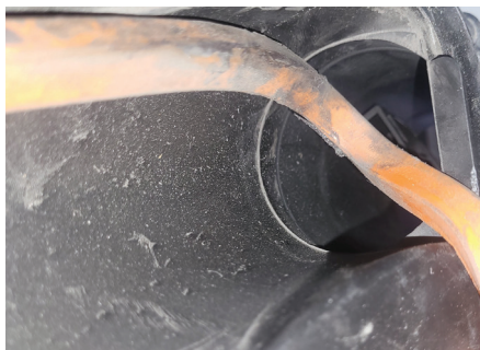
The loose portion of the air filter was interfering with the mass flow sensor
