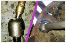
Both the inner and outer track rod joints were worn
