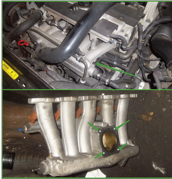
The throttle body sits below the manifold and can only be accessed once the manifold is off
