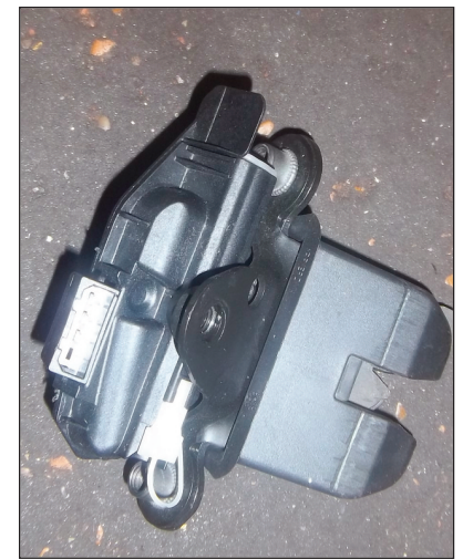
The rear hatch catch is electrically operated and has no mechanical connections
