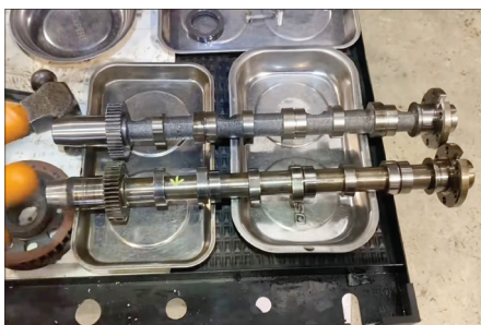
When compared to a new camshaft, the old cams were noticeably out of position
