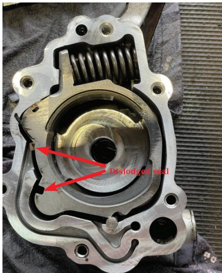
A dislodged apex seal had jammed the pump
