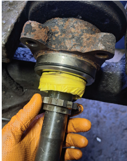
Cover the teeth of the sensor ring to protect them from foreign objects
