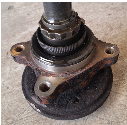
The wheel bearing and ABS sensor ring are held in place with a crimped nut threaded onto the axle shaft
