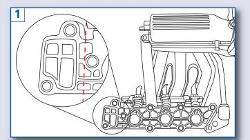
Once removed from the car, hold or carefully clamp the plastic inlet manifold. Mark the coolant blanking section of the manifold that you are about to saw through, making sure that you mark a section slightly larger than the size of the new blanking plate. This is to ensure there is no interference between the manifold and new blanking plate when they are fitted to the engine. Check twice – cut once!
