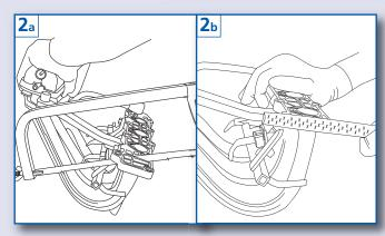
Plug the three outlet ports to prevent debris falling into the manifold. Carefully saw through the manifold and remove the old blanking section. Then trim/file the rough edges of the manifold to ensure a flat mating surface is maintained and clean as necessary
