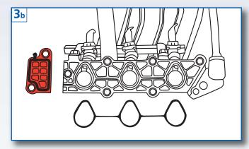
Ensure that the mating surface of the cylinder head is clean and refit the manifold using the new manifold gasket supplied. Fit the new blanking plate onto the cylinder head, using a little RTV if required. Tighten all manifold nuts to the manufacturer's specifications. (15-19Nm)
