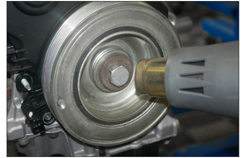
Carefully heat the bolt with a hot air gun
