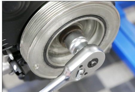
Never use an impact wrench on a pulley bolt
