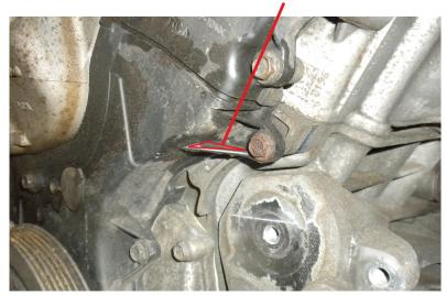
IMPROPER INSTALLATION MAY RESULT IN A DAMAGED FRONT TIMING BELT COVER AND IMPROPER ACCESSORY BELT TRACKING, EVENTUALLY LEADING TO BELT FAILURE!
