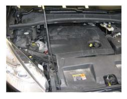
The engine cover must be removed for the low-pressure side to be connected.
