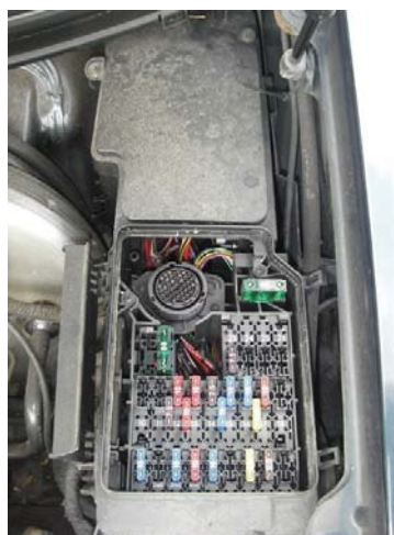
W210 fuse and relay box
