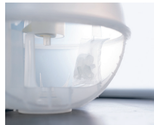
Figure 1: Coolant expansion tank with silica gel bag
