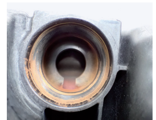
Figure 2: Deposits in the coolant expansion tank
