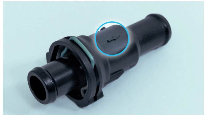
Figure 1: Always note the installation direction (marked with an arrow) when installing the thermostat.
