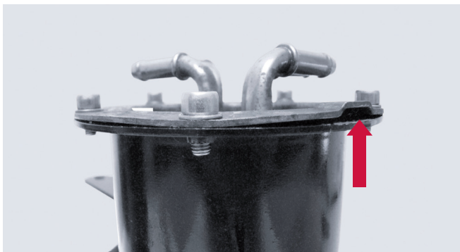
Figure 1: Correct point for levering off the cover
