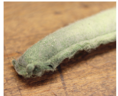
Worn out receiver dryer (or desiccant bag cartridge) often results in clogging of the condenser's inner tube
