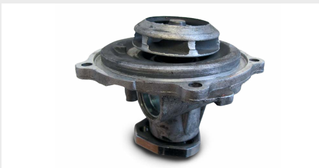
Bearing damage due to excess belt tension
