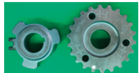
The fuel pump sprocket (right) can rotate freely from the separate base section (left)
