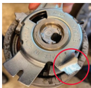
A tensioner that was damaged by incorrect tensioning
