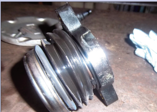
The collapsed DMF allowed the concentric slave cylinder to extend past its intended travel, until it started to leak
