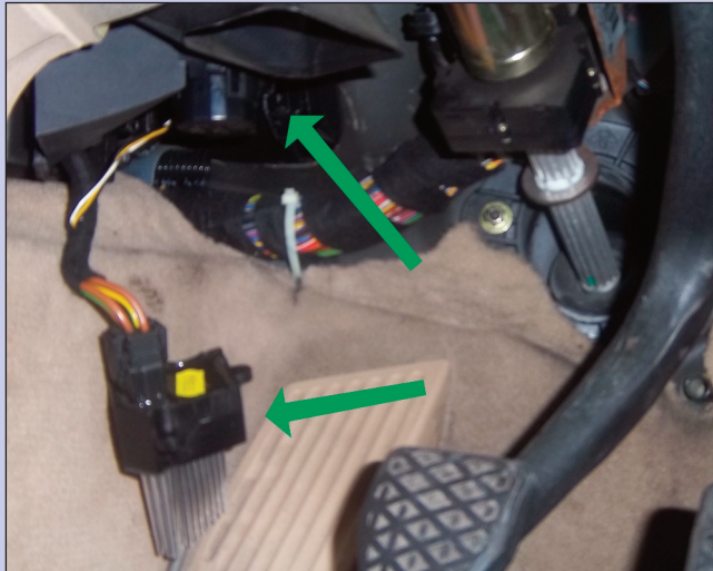
The hedgehog is fitted up under the driver's footwell with limited, but not impossible access
