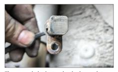
The expanded reluctor ring had worn into the road speed sensor, causing the ABS fault
