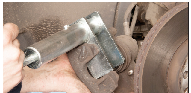
Retracting the brake piston
