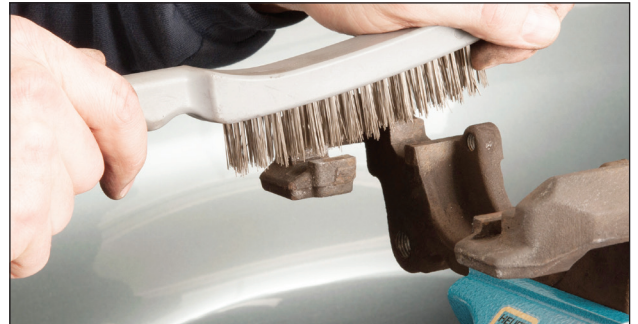
Derusting mounting and guide surfaces
