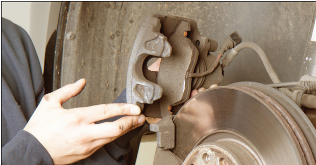
Removing the brake pads
